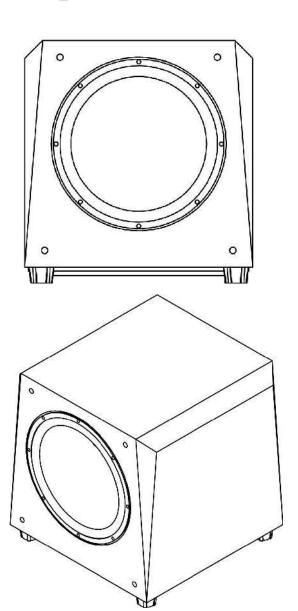
System Type: Subwoofer, pneumatically coupled
