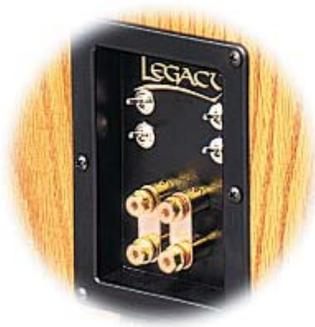
Connect each channel of your amplifier to a loudspeaker via the five-way gold binding posts provided. Dual banana plugs or gold plated spade lugs are recommended means of termination. Be sure that you observe polarity when making the connections. The positive (+) terminal of the amplifier should be connected to the positive terminal of the loudspeaker. The negative (-) terminal of the amplifier should be connected to the negative terminal of the loudspeaker.
