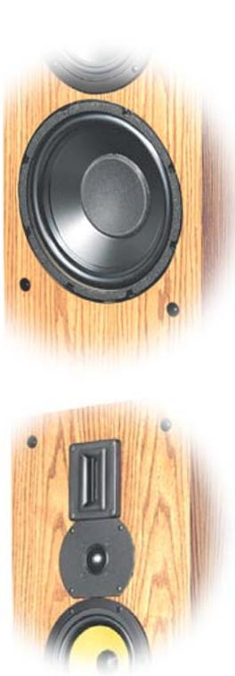
The Signature loudspeakers dedicate dual 10" carbon-filled bass drivers with a total of 20 pounds of motor structure and a free air resonance frequency of 18 Hz. The midbass is picked up by an ultra-quick 7" Kevlar® Hexacone with graphite frame and a 7" curvilinear polypropylene driver with a vented pole piece and cast magnesium basket. The dust cap is covered with a soft PVC nose to prevent secondary radiation. A butyl rubber surround assures linearity.
